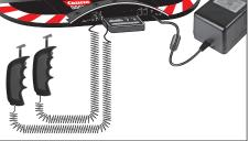
Connect the transformer plug with the Control Cont.
