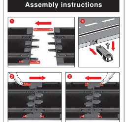
**()** + **(2)** + **(3)** Before assembling please insert the connecting clips in the track as shown in figure **()**. Stick tracks together on a flat base. Move the connecting clips according to figure 2 in direction of the arrow until they audibly snap in. The connecting clip may also be inserted later. The connecting clips can be removed into both directions by simply pressing down the clamped nose (see fig. 3).
