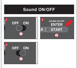
The confirmation sound when crossing the sensors and the key sound can be switched off. Switch off the Control Unit and keep the "START/ENTER" button (3) pushed, switch on the racetrack and release "START/ENTER" (3) again. The acknowledgement sound for switching on the Control Unit cannot be switched off however.
