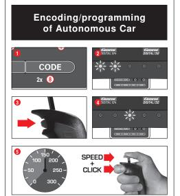
Switch on the Control Unit, place the car to be encoded on the track and press "Code" (8) twice, fig. (1). The first two LEDs at the Control Unit start to light, fig. (2). Now push the lane-change button at the speed controller, fig. (3); LEDs 3-5 will light successively. Wait until the middle LED lights again, fig. (3). Activate the speed controller's tappet until the car has reached the desired speed. Now push lane-change button again, fig. (5). Autonomous Car's encoding is completed now.
