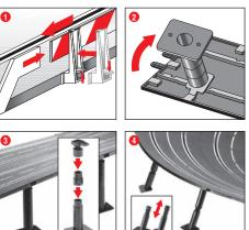
**Guard rails:** Guard rail mounts are fitted by tilting them upwards onto the verge of the track.
