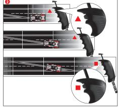
Make sure that the car's guide keel is located inside the track slot and that the double sliding contact is in contact with the current carrying track.
