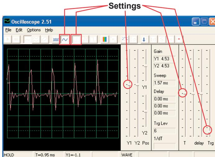
**Note:** Although the amplitude of the pulses appears to be varying across the screen (the wider time scale shown below shows this better), this is an illusion caused by the way Winscope measures the signal. The amplitude of the pulses is not really varying.
