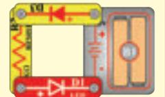
27. **SCR (Q3):** Build the mini-circuit shown here. Turn on the slide switch (S1) and the motor (M1) should not spin. Press the press switch (S2), the motor should start spinning. Now turn the slide switch off and on, the motor should not spin.
