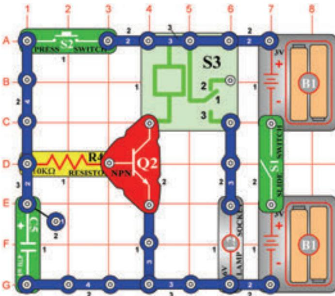
The transistor (Q2) acts as a switch, connecting the relay (S3) to the batteries. As long as there is positive voltage on the transistor's base, the bulb (L2) will light.
