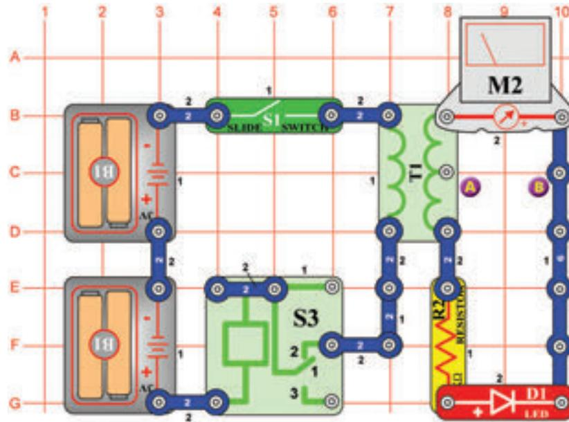
**OBJECTIVE:** To build a half wave rectifier circuit.
