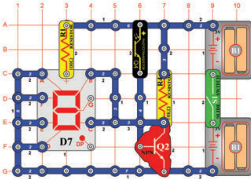
**OBJECTIVE:** To make a circuit that indicates whether a door is open or closed.
