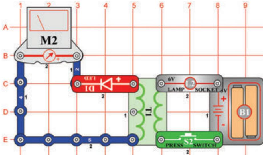
Set the meter (M2) to the LOW (or 10mA) scale. Pressing and releasing the press switch (S2) continuously generates an AC (changing) current. The LED (D1) is used to convert the AC (changing) current to DC (unchanging) current because it only allows the current to flow in one direction. The LED should light as the meter deflects to the right only. Without the LED, the meter would deflect in both directions.
