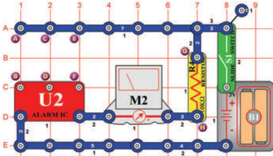
**OBJECTIVE:** Use the meter with the alarm IC.
