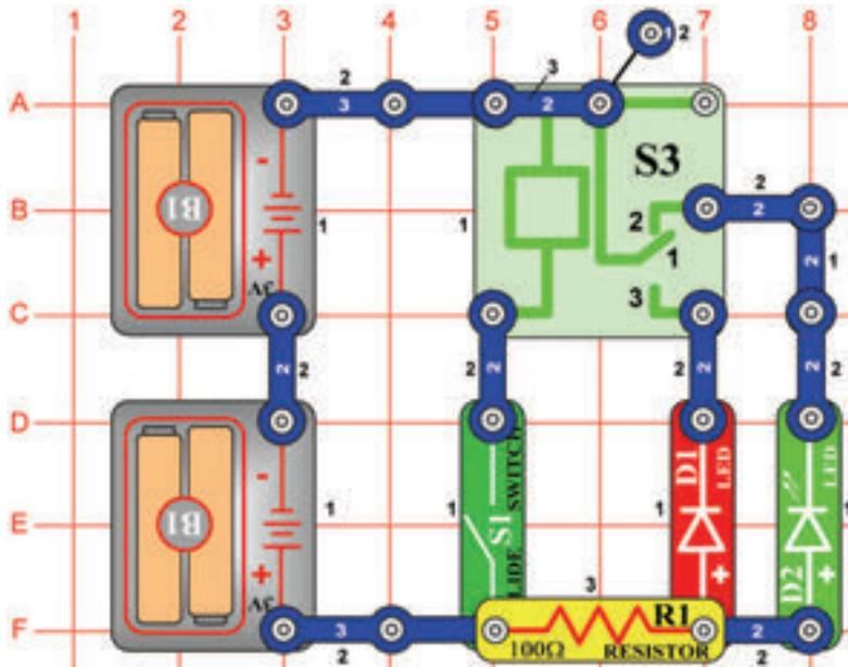
A relay is an electronic switch with contacts that are opened or closed using voltage. It contains a coil that generates a magnetic field when a current flows through it. The magnetic field attracts an iron armature which switches the contacts. Contact #2 is normally closed, connecting the green LED (D2) and the resistor across the batteries.
