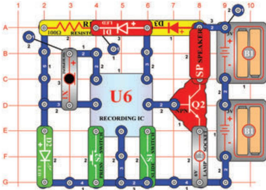
**OBJECTIVE:** To build a circuit that lights an LED to indicate the recording mode.
