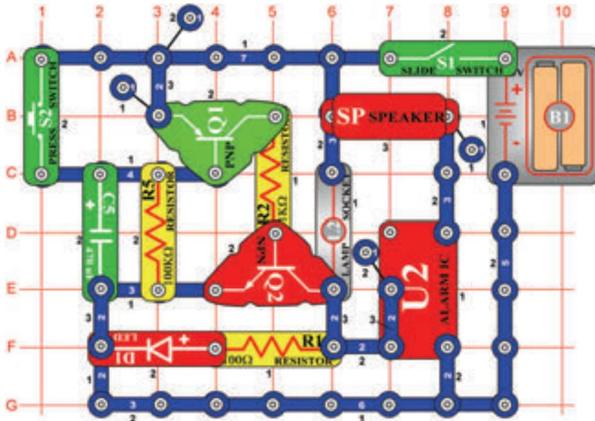
Turn on the slide switch (S1) and the alarm may sound and slowly drift away as the lamp (L2) brightens. Press the press switch (S2) and the alarm sounds at full volume as the LED (D1) lights. Capacitor C5 is also charged. Release the press switch; the alarm IC (U2) still sounds because the voltage from the discharging C5 keeps Q1 and Q2 off. As the capacitor's voltage drops, the LED will turn off and the sound will slowly stop.
