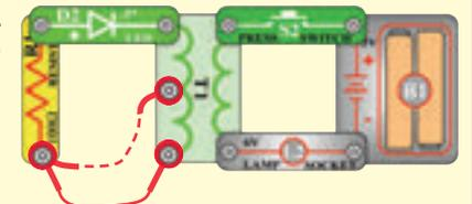
26. **Diode (D3):** Build the mini-circuit shown here, the red LED (D1) should light. Reverse the direction of the diode, the LED should not light now.
