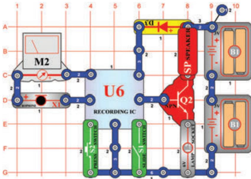
**OBJECTIVE:** To add a volt meter to the playback and record circuit.
