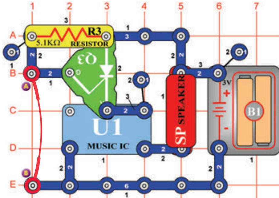
The alarm circuit activates when you remove the jumper wire from points A & B. The jumper wire shorts the SCR's (Q3) gate to ground and the SCR does not conduct. Removing the jumper wire places a voltage on the gate and the SCR conducts. This connects the battery to the music IC (U1) and music is played.
