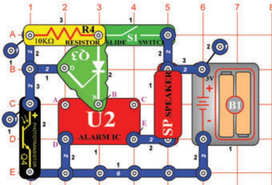
As the phototransistor (Q4) is exposed to light, its resistance is very low, thereby connecting the gate of the SCR (Q3) to ground. This prevents the SCR from conducting, connecting the alarm IC (U2) to the batteries. The alarm IC remains off until the light is blocked, triggering the SCR. If the light in the room is not bright, the IC may turn on.
