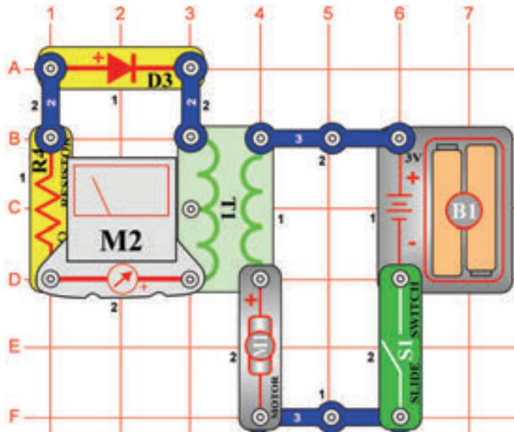
Set the meter (M2) to the LOW (or 10mA) setting. By placing the meter, diode (D3) and current limiting resistor (R4) on the transformer (T1), you can measure the current. Turn on the slide switch (S1) and the motor (M1) starts spinning. The current on the right side of the transformer creates a current on the left side using magnetism.
