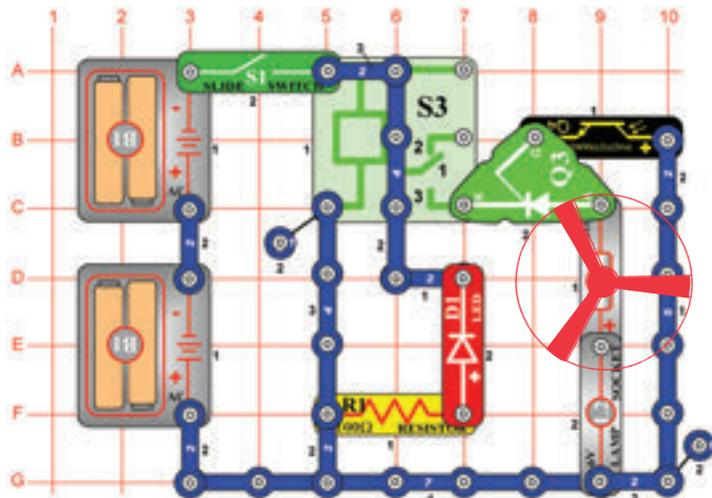
Cover the phototransistor (Q4) with your finger. Turn on the switch (S1), and only the LED (D1) lights. The relay (S3) connects the motor (M1) and the bulb (L2) to the batteries, but the motor and bulb are powerless until a voltage is applied to the SCR's gate.
