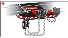
The connecting rail is the straight track with sockets for the transformer and hand-held control unit.
