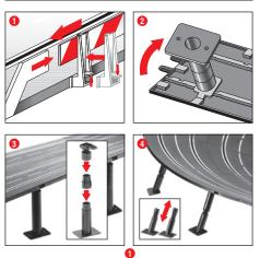
Guard rails: Guard rail mounts are fitted by tilting them upwards onto the verge of the track.
