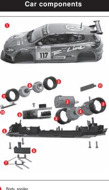
000 Body, spoiler Engine Tyres Rear axle Chassis Guide keel Double sliding contact Front axle Car board with reversing switch Front light board Ā Rear light board
