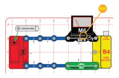
Build the circuit shown. Set the meter (M6) to the 50mA setting. Push the press switch (S2) and watch the current on the meter when the crank arm on the geared motor (GM) spins.
