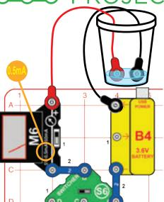
Build the circuit, set the meter (M6) to the 0.5mA setting, and set the switcher (S6) to he right position. Add about 1/4 inch of water to a cup or bowl. Connect the jumper wires to the circuit as shown and place the loose ends in the water, make sure the metal parts aren't touching each other. Measure the current through the water.
