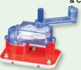
The **geared motor (GM)** is a motor with a gearbox attached. The crank arm may be attached to it so it can be turned by hand. The gearbox spins the motor shaft faster but with less force than when turning the crank arm.
