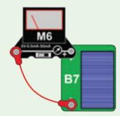
3. Snap wires: Set the meter to the 5V setting and use this circuit to test each snap wire, one at a time. Place the solar cell (B7) near the same light source you used in step 1. The snap wire is damaged if the meter pointer does not move.
