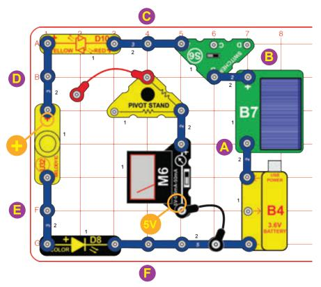
Build the circuit and set the meter (M6) to the 5V setting. Connect the black jumper wire between the meter and 5-snap wire. Connect one end of the red jumper wire to the pivot stand; leave the other end loose. Set the switcher (S6) to the left position. Place the solar cell (B7) in bright sunlight or near an incandescent lamp. If the light is bright enough, the LEDs (D8 & D10) will light and the melody IC will make a little noise.
