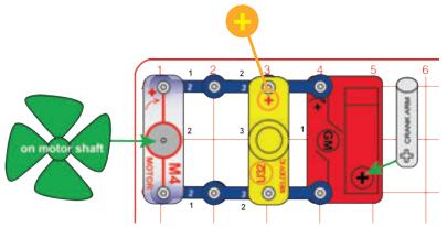
Turn the crank arm clockwise to run the fan and melody IC (U32).
