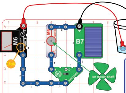
Build the circuit, place the wind fan on the motor (M4), and set the meter (M6) to the 0.5mA scale. Place the circuit so wind is blowing on the fan or sunlight is shining on the solar cell (B7). Set the switcher (S6) to the left position if you have wind or to the right position if you have sunlight. Connect the jumper wires to the circuit and place the other ends in a cup of water, make sure the metal parts aren't touching each other.
