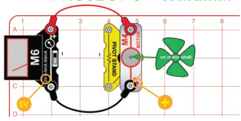
Assemble the pivot stand, mount the wind fan on the motor (M4), mount the motor on the pivot, place the pivot on the base grid and connect it to the meter (M6) using the red and black jumper wires. Set the meter to the 5V setting.
