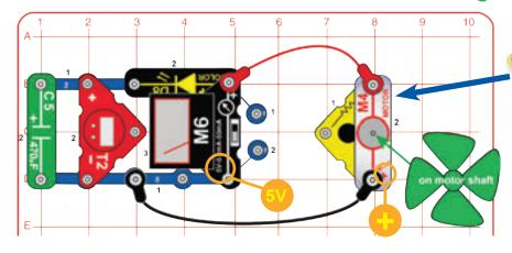
Build the circuit shown. Set the meter to the 5V setting. Blow on the fan or place it in a strong wind (either outside or near an electric fan). The meter (M6) measures how much voltage your "windmill" produces. You may need to give the fan a push to get it started.
