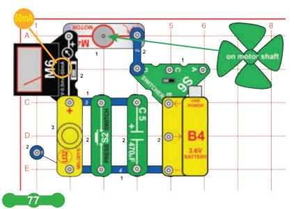
Set the meter (M6) to the 50mA setting, and set the switcher (S6) to the left position. You should hear a beeping sound from the melody IC (U32) as the meter measures the current. Spin the fan in either direction with your finger to change the sound. Push the press switch (S2) to spin the fan.
