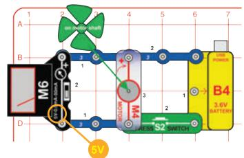
Modify the preceding circuit into this one. Set the meter (M6) to the 5V setting and place the wind fan on the motor (M4). Push and release the press switch (S2) and watch the voltage on the meter as the motor speeds up and slows down.
