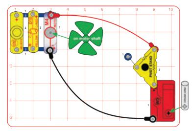
Turn the crank arm on the geared motor (GM) clockwise to run the motor (M4) and fan, red/yellow LED (D10), and melody IC (U32) or turn it backwards to run iust the motor and LED.
