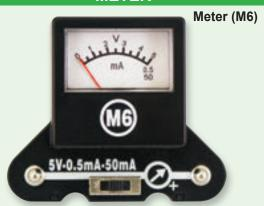
The **meter (M6)** is an important measuring device. You will use it to measure the voltage (electrical pressure) and **current** (how fast electricity is flowing) in a circuit.
