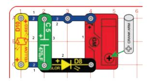
Turn the crank arm clockwise to light the LEDs (D8 & D10). Turn the crank at a constant speed so both LEDs light, and notice how now the red/yellow LED brightness does not vary as much.
