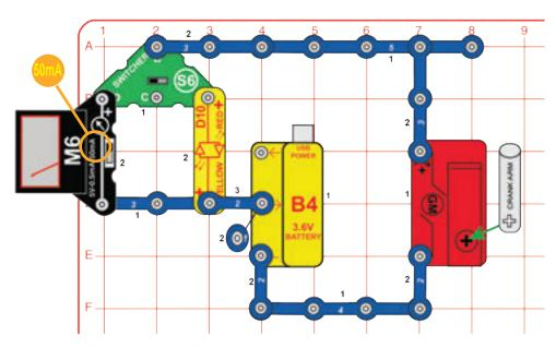
Use the crank arm to charge the battery (B4), the meter (M6) or LED (D10) show how fast you are charging it.
