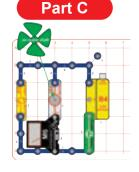
Build the circuit and set the meter (M6) to the 50mA setting. Push the switch (S2); the meter measures the current from the battery (B4). let the fan get to full speed.
