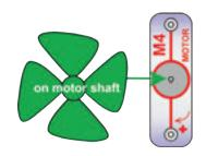
In the preceding circuit, replace the color LED (D8) with the motor (M4, in either direction) and place the wind fan on it. Now press the switch and watch how the voltage changes as the solar cell runs the fan. Depending on your light source, the fan may need a push to get started or may not work at all.
