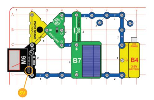
Build the circuit shown. Place the solar cell (B7) in sunlight or close to an incandescent lamp. Set the meter to the 5V setting, but double the reading it shows, since a resistor in the pivot stand converts the scale to 10V. If the switcher (S6) is set to the upper position, then the meter shows the battery (B4) voltage. If it is set to the lower position, then the meter shows the solar cell (B7) voltage.
