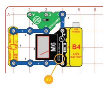
Build the circuit and set the meter (M6) to the 5V setting. Set the switcher (S6) to the right position and watch the voltage on the meter for a while as the battery runs the red/yellow LED (D10). How quickly does the voltage drop?
