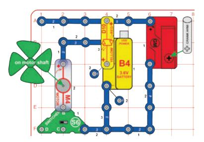
Set the switcher (S6) to the left position and turn the crank arm on the geared motor (GM). The LED (D10) lights when the crank is charging the battery (B4).
