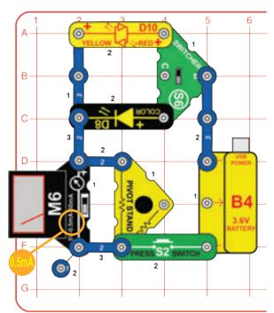
Build the circuit shown. Set the meter (M6) to the 0.5mA setting.
