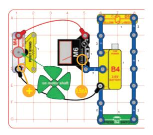
Build the circuit shown. Set the meter (M6) to the 0.5mA setting. Blow hard on the fan or place it in a very strong wind (either outside or near an electric fan). The "windmill" charges the battery (B4) when the wind is blowing hard, and the meter measures the charging current. Push the press switch (S2) to turn on the LED (D10).
