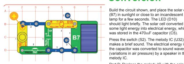
The capacitor stores energy as an electric field, similar to the magnetic field of a magnet. It can only store a small amount of energy in this way.
