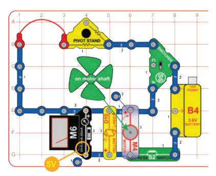
Set the switcher (S6) to the top or bottom position and push the press switch (S2); the motor (M4) spins the fan, the LED (D10) lights, and the meter (M6) measures the voltage across them.
