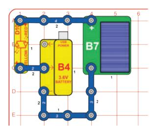
This circuit uses the solar cell (B7) to charge the rechargeable battery (B4). Place the solar cell in sunlight or near an incandescent light bulb. The red/yellow LED (D10) lights red when the battery is being charged. The brighter the LED, the faster it is charging.
