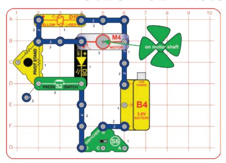
In this circuit we use the LED's (D8 & D10) to indicate if the motor (M4) is spinning. Set the switcher (S6) to the left position, the color LED lights, indicating the motor is not spinning. Pushing the press switch (S2) bypasses the color LED, and it turns off. The voltage across the motor and red/yellow LED increases, so they turn on.
