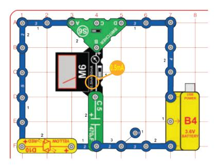
Build the circuit shown. Set the meter (M6) to the 0.5mA setting. Flip the switcher (S6) back and forth between its left and right positions to charge and discharge the 470mF capacitor (C5).
