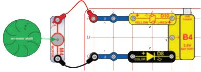
Place the water wheel on the motor (M4) and connect it to the circuit as shown. Hold the motor under a water faucet so the water wheel will "catch" the water as it falls. The LEDs (D8 & D10) should light.
