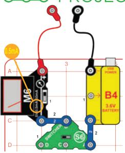
Build the circuit, set the meter (M6) to the 0.5mA setting & set the switcher (S6) to the right position.
