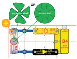
Build the circuit, and place either the wind fan or the water wheel on the motor (M4). To make the LEDs (D8 & D10) bright, blow on the wind fan from above, or blow into the "curves" of the water wheel.
