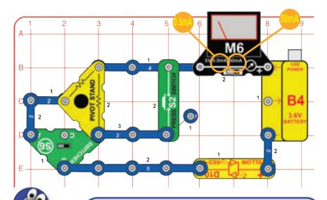
Adding resistors to a circuit is like partially blocking a water pipe, reducing the flow of water.
