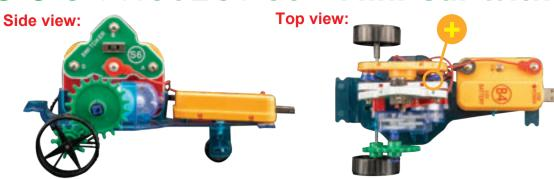
Use the project 34 circuit but add the melody IC (U32) using two 1-snap wires, as shown. A tune plays when the car moves backward. You can reverse the orientation of the melody IC to make the sound play when the car moves forward.
