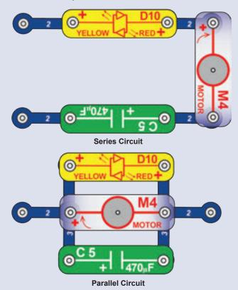
Placing components in series increases the resistance; highest value dominates. Placing components in parallel decreases the resistance; lowest value dominates.
