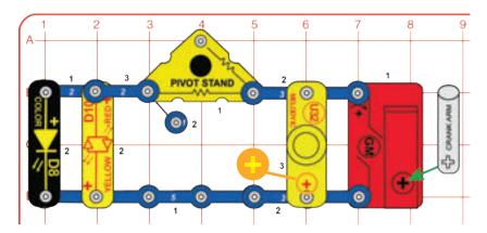
Turn the crank arm on the gearedmotor (GM) slowly clockwise, just enough to turn on the red/yellow LED (D10, which will be red) and make the color LED (D8) show red. Then crank faster, until the color LED also shows green and blue brightly.
