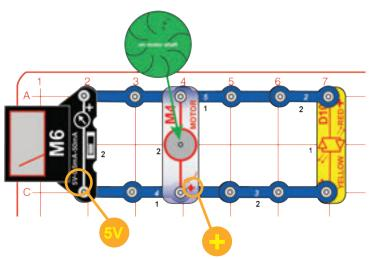
Build the circuit as shown, with the water wheel on the motor. Set the meter (M6) to the 5V setting. Blow on the water wheel, aiming the air into the "curves" on the fan. Watch the meter to see the voltage produced, and the red/yellow LED (D10) will light red.
