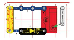
Turn the crank arm clockwise to light the LEDs (D8 & D10). Turn the crank at a constant speed so both LEDs light, and notice how both are flashing.
