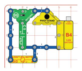
The electrons slowly trickle into the  $470 \mathrm{mF}$  capacitor (C5) through a  $10 \mathrm{KW}$  resistor (in the pivot stand) when the switcher (S6) is in the right position. If you wait and let the capacitor charge up it will flash nicely when you switch to the left. If you are not patient, and switch back too quickly your flash will be weak.
