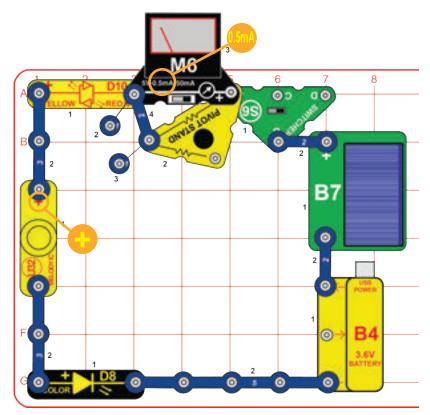
the 0.5mA setting. Set the switcher (S6) to the left position. Place the solar cell (B7) in bright sunlight or near an incandescent lamp. If the light is bright enough, the meter will show a current, the LEDs (D8 & D10) will light, and the melody IC (U32) will make a little noise.
