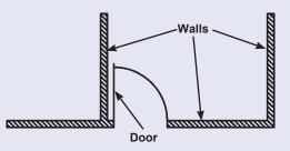
The electronics symbol for a simple switch should be thought of as a door to a circuit, which swings open when the switch is off. The "door" to the circuit is closed when the switch is on. This is shown here:
