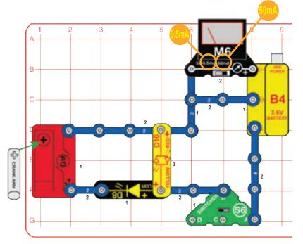
Build the circuit by setting up the parts as shown. Set the meter (M6) to the 0.5mA or 50mA setting. Set the switcher switch (S6) to the right position to connect the rechargeable battery (B4) to the red/yellow LED (D10). If the battery is charged, the LED will light and the meter will show that an electric current is flowing out of the battery. The 0.5mA meter scale will show a high current while the 50mA scale may show little or no current.
