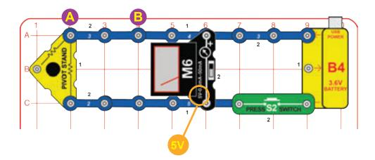
Modify the preceding circuit to be this one, which connects to a different resistor in the pivot stand. Set the meter (M6) to the 5V setting and push the press switch (S2). Read the voltage on the meter.
