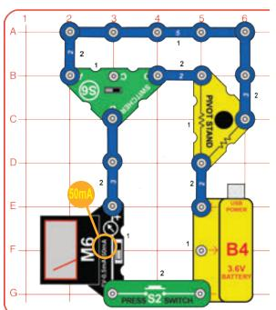
Build the circuit shown. Set the meter (M6) to the 50mA setting and the switcher (S6) to the right position. The pivot stand base has 47W and 10KW resistors in it. They are used to control the flow of electricity in a circuit.
