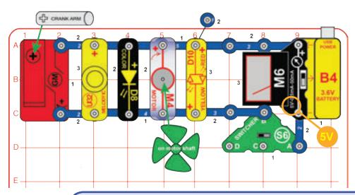
Build the circuit and set the meter (M6) to the 5V setting. Set the switcher (S6) to the left or middle position (off) and read the battery (B4) voltage when it is not running anything.
