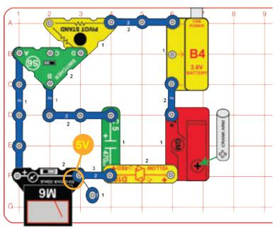
The  $470 \mathrm{mF}$  capacitor (C5) is a storage device, so it would be nice to know when it is filled to capacity. With the switcher (S6) in the right position, turn the crank arm until the LED (D10) no longer produces light. When the capacitor is fully charged, the current is blocked and the light cannot turn on.
