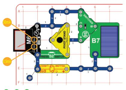
Build the circuit shown. This circuit measures current using several scales on the meter (M6). Set the switcher (S6) to the top position. Place the solar cell (B7) in sunlight or near an incandescent lamp, and vary the light on it. Use the 0.5mA or 50mA settings on the meter to measure the current through the LED (D10).
