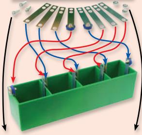
Connect the 3 electrode parts together with screws and nuts as shown. Tighten by hand, a screwdriver is not needed.
