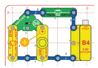
Build the circuit shown and push the press switch (S2) to turn on light or sound. Switches can be arranged in many different ways.
