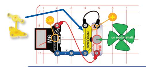
Build the circuit as shown, with the motor (M6) on the pivot and the wind fan on the motor. Set the meter (M6) to the 50mA setting. Blow on the fan or place it in a strong wind.
