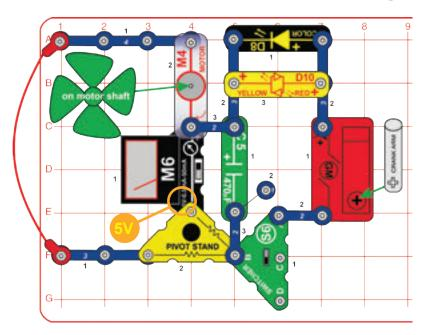
Set the switcher (S6) to the top position and turn the crank arm on the geared motor (GM). The LEDs (D8 & D10) light, the meter measures the voltage, and the fan spins.
