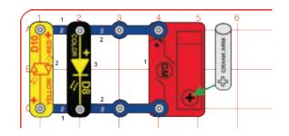
Turn the crank arm clockwise to light the LEDs (D8 & D10). Turn the crank at a constant speed so both LEDs light, and notice how only the color LED is flashing now.
