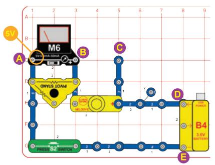
Build the circuit and place the wind fan on the motor (M4). Set the meter (M6) to the 5V setting. Push the press switch (S2); the meter measures the voltage across a resistor in the pivot stand. The measured voltage varies a little as the sound changes.
