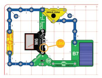
Build the circuit shown. Set the meter (M6) to the 0.5mA setting. Set the switcher (S6) to the right position, place the solar cell (B7) in sunlight or near an incandescent lamp, and push the press switch (S2). The solar cell slowly charges up the  $470 \,\mathrm{mF}$  capacitor (C5), and the meter shows the current.
