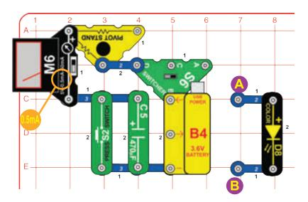
Set the meter (M6) to the 0.5mA setting, and set the switcher (S6) to the left position. Watch the current on the meter as the  $470 \mathrm{mF}$  capacitor (C5) slowly charges up. Once C5 is near full charge you can push the press switch (S2) to instantly discharge the capacitor and restart the charging process.
