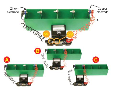
Assemble the liquid energy source using the instructions on page 4. Connect the red & black jumper wires between the meter (M6) and the electrodes, the (+) side of the meter goes to the copper one. Set the meter to the 5V setting. Fill the compartments with cola soda (other flavors also work). The meter should show a voltage of about 3V. Switch the meter to the 0.5mA setting to measure the current produced.
