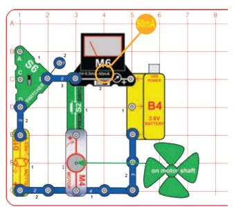
Build the circuit and set the meter (M6) to the 50mA setting and the switcher (S6) to the top position. Set the switcher to the bottom position to measure the current through the LED (D10), push the press switch (S2) to measure the current through the motor (M4), or do both to measure the combined current.
