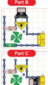
Build the circuit and set the meter (M6) to the 5V setting. Push the switch (S2); the meter measures the voltage across the motor. The voltage increases as the motor speeds up.
