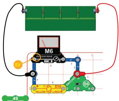
Connect the liquid energy source to the circuit shown here. Fill the compartments with water. Set the switcher (S6) to the left position. Set the meter (M6) to the 5V setting to see the voltage produced. The red/yellow LED (D10) may be dimly lit, depending on your local water supply. If you set the switcher to the right position, the voltage may be higher since the water is not trying to light the LED.
