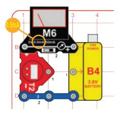
Build the circuit shown. Set the meter (M6) to the 0.5mA setting. The clock display will light, but the meter will not measure any current. See page 4 if you would like to set the time.
