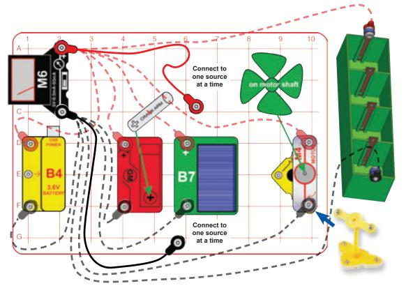
Boffin has 6 electrical power sources: battery, hand crank, solar cell, windmill, watermill, and liquid holder. Let's compare them. The watermill is similar to the windmill and its messy, so we'll skip it.
