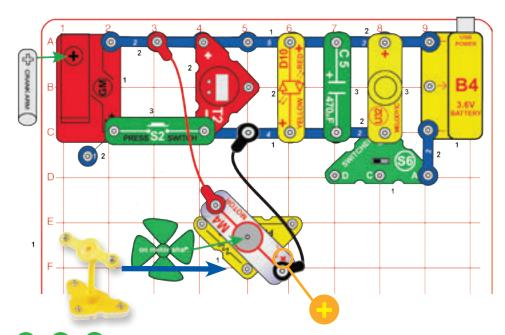
Make sure the battery is charged up (see project 3). Build the circuit with the motor and fan on the pivot stand, and connect the jumper wires as shown. Set the switcher (S6) to the right position to turn on the circuit. The battery runs the clock display (T2), melody IC (U32), red/yellow LED (D10), and windmill (M4). Push the press switch (S2) and the crank arm on the geared motor (GM) will also spin.
