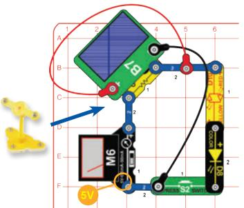
Assemble the pivot, mount the solar cell (B7) on it, and place it in the circuit as shown. Connect the solar cell to the circuit using the red and black jumper wires. Place the circuit so the solar cell is in bright sunlight or close to an incandescent light bulb. Set the meter (M6) to the 5V setting.
