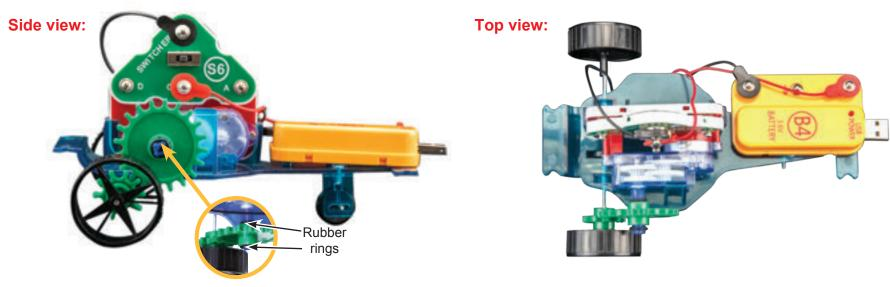
Build the circuit as shown, initially setting the switcher (S6) to the middle setting. Mount the 1.75" gear on the geared motor (GM) with the rubber rings to keep it from sliding out of position, place it on the mini car frame, and connect the battery (B4), switcher (S6) and red & black jumper wires as shown. Use the switcher to make the mini car go forward, backward-turning, or stop.
