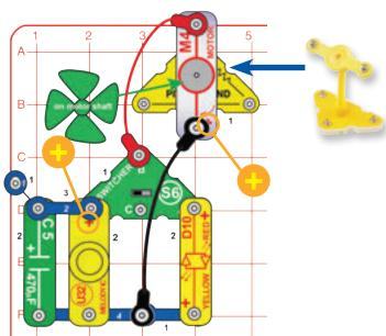
Build the circuit as shown, with the motor on the pivot stand. Set the switcher (S6) to the left for sound (in one wind direction) or to the right for light. Blow on the fan, place it in a strong wind, or give it a good spin with your fingers. The fan must spin very fast to produce sound.
