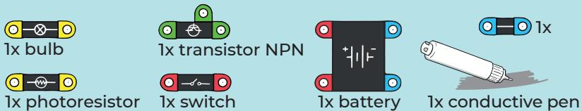
The more the photoresistor is illuminated, the more light the bulb emits since the transistor opens. The build is functionally the same as LL160, however the direct series combination of a photoresistor and bulb would have such a high resistance that the bulb would not light up on battery power. That is why we will use the transistor as a voltage amplifier for the bulb.
