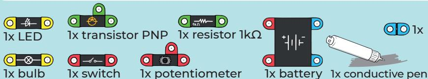
Use a potentiometer to control the current flowing through a LED diode to the transistor base. However, the LED is in the reverse direction, and so no current flows through the base and there is nothing to amplify. The bulb cannot light up because the transistor is closed.
