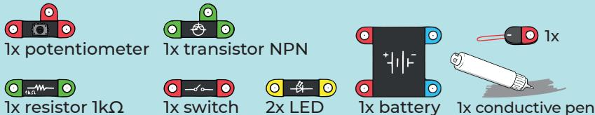
The circuit demonstrates the ability of a transistor to amplify the electric current. Use a potentiometer to control the current flowing through LED diode to the transistor base. A low current that is barely sufficient to turn on the LED will cause the transistor to open to the extent that the voltage on the LED is sufficient to light it up.
