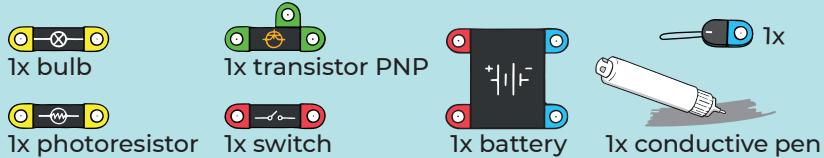
Functionally, this is the same build as LL550, but with a transistor of opposite conductivity. The direction of the base current is opposite, so it is necessary to modify the base circuit. The bulb is connected in the emitter circuit (see LL460), so the bulb reacts with lower brightness because the voltage on the bulb is low as it copies the voltage on the photoresistor.
