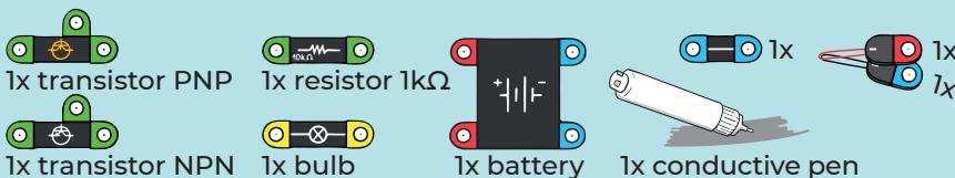
Using a pair of transistor amplifiers, we can turn on the light bulb also with a touch button. With the NPN transistor, we amplify the contact current through the button and we amplify it again with the PNP transistor. When the button is touched, the bulb lights up at full brightness, as if it were connected directly to the battery.
