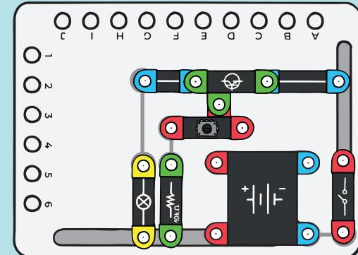
By changing the low current to the transistor base, you can control the high current flowing through the bulb since opening and closing the transistor causes the voltage on the bulb to change. We use an NPN transistor in this case.
