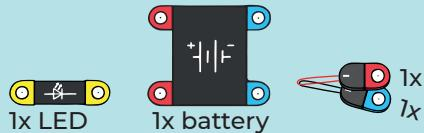
The basic electrical circuit can be used directly as a conductivity detector. If the object is conductive, i.e. it is able to conduct electric current, the conductive object is indicated by the LED light. Since a relatively small current is enough to light up the LED, we can even detect the less conductive objects. The best result is achieved by using a white LED diode, which has a high brightness and even its low light is so noticeable.
